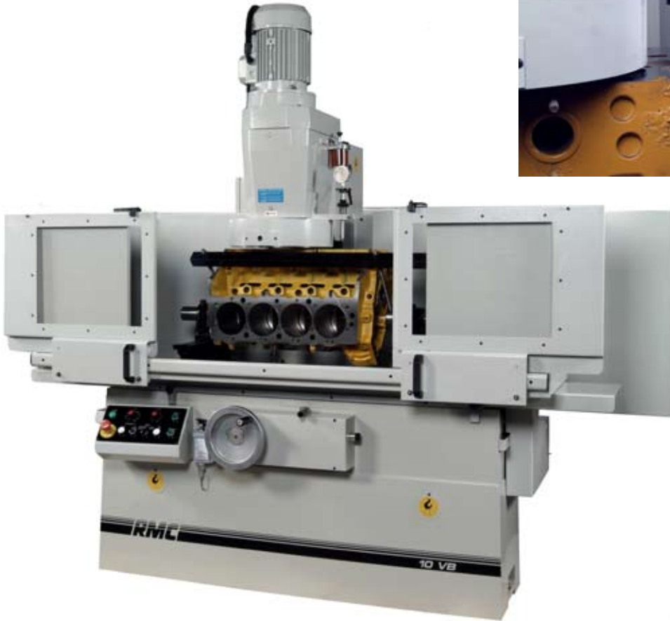
RMC's optional quick mounting and leveling rolover fixture lets you surface most passenger car and medium size diesel heads and blocks.
