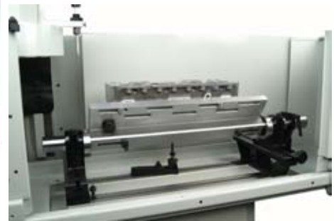
RMC's optional quick mounting and leveling rolover fixture lets you surface most passenger car and medium size diesel heads and blocks.
