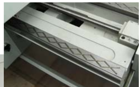
RMC's optional quick mounting and leveling rolover fixture lets you surface most passenger car and medium size diesel heads and blocks.
