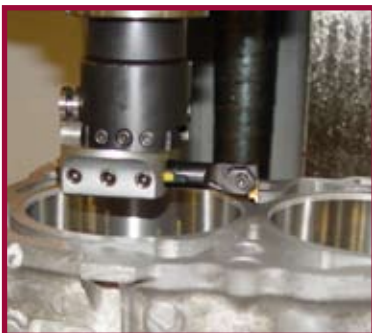
O-ring grooving and Cylinder bore chamfering
