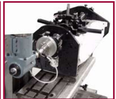
Line and Cam Tunnel Boring
