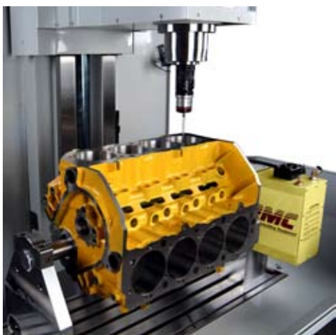
RMC's digital probe option is a one step process for premachining block checking of bore diameters, locations and deck heights. Measurements will appear on screen for operator verification.
