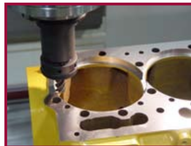
Circular interpolation of Counterbore
