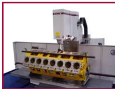
Lower Sleeve Repair
